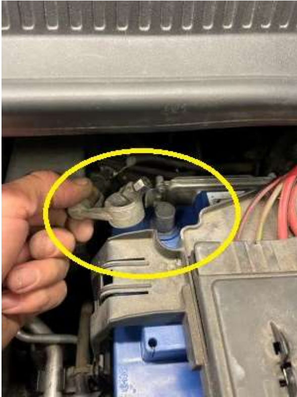
Undo the minus from the battery
