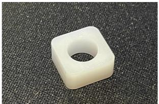
Slide off the old worn plastic guide bush from the shaft.
