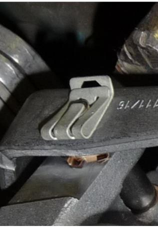
Locate the small metal retaining clip on the selector mechanism.
