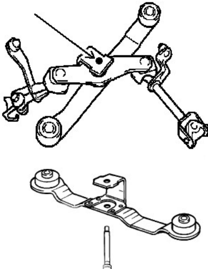
**Dismantle the old linkage complete and reassemble every part on the new linkage (or shift shortener)** When re-assembling , fill everything with silicone grease before fitting to be sure of a smooth gearchange.
