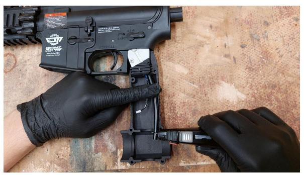
Cut the 6mm macroline equally with the compartment for the regulator  $% \left( 1\right) =\left( 1\right) \left( 1\right$
