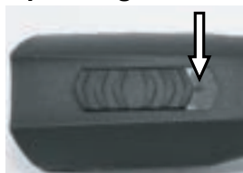
Fig. 4 Switch in OFF-position ("0")
