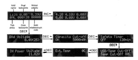
During charging, the charger program allows you to view the pre- defined operating parameters of the device and view the current voltage on individual cells. Using the DEC/INC buttons, it will be possible to switch between subsequent screens with the following indications:
