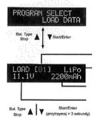
Use the BATT TYPE/STOP button to select the LOAD DATA option and confirm your selection with the START/ENTER button.
