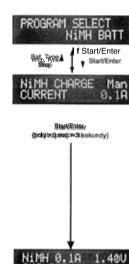
Using the BATT TYPE/STOP button, we select the battery program appropriate for the given type of nickel batteries (NiCD/NiMH), and confirm with the START/ENTER button.
