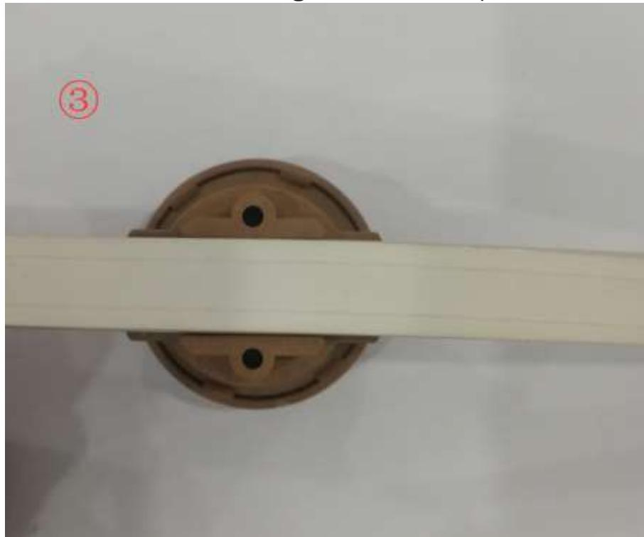
4. Place the smaller part (the base) of the lamp holder on top.
