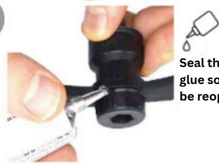
Seal the connection with glue so the fitting cannot be reopened.
