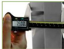
75 mm insulation thickness
