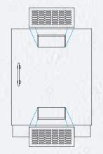
**Front Ventilation** Cut ventilation grilles into a standard door panel.
