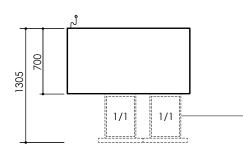
Fully extendable drawers suitable for 100mm deep gastronorm pans. The pan top lip maximum height should be no more than 5mm.
