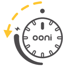
Push, slowly turn and hold for 3 seconds to light. Hold in for another 5 seconds after ignition.
