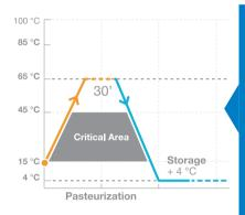
With the automatic **self-pasteurization (optional only for XVL 1 and XVL 3)** system you can choose when to wash the machine up to a maximum interval of 42 days. As a further guarantee of hygienic safety, if the operator does not perform the complete cleaning at the end of the set days, the machine goes into automatic block.
