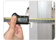
80 mm thick eco-friendly insulation
