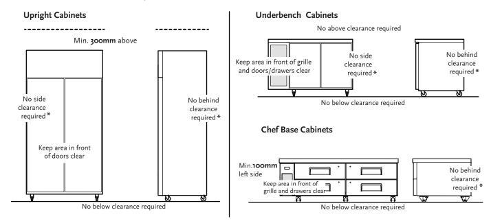
\*When installed for continuous duty in climate class 7 environment (35°C ambient / 75% relative humidity), it is recommended to provide 50mm clearance around the sides and back of the cabinet.
