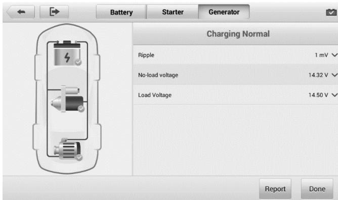
**Figure 10-10 Sample Generator Test Results Screen**
