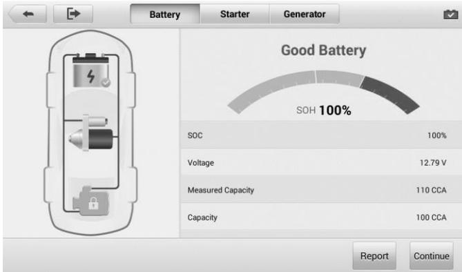
**Figure 10-7 Sample Battery Test Results Screen**
