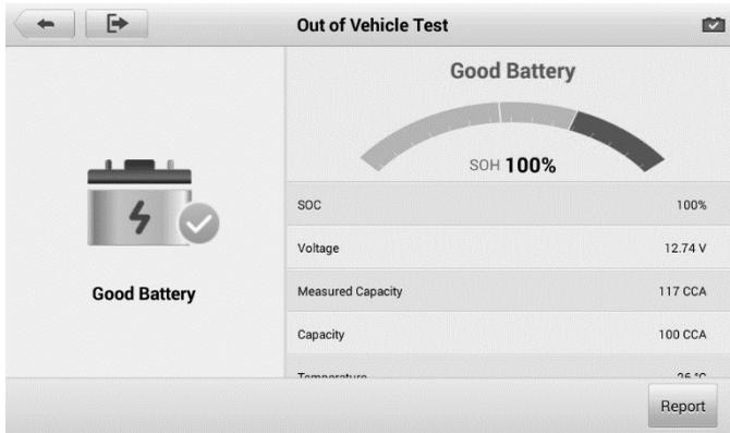
**Figure 10-12 Sample Out of Vehicle Test Results Screen**
