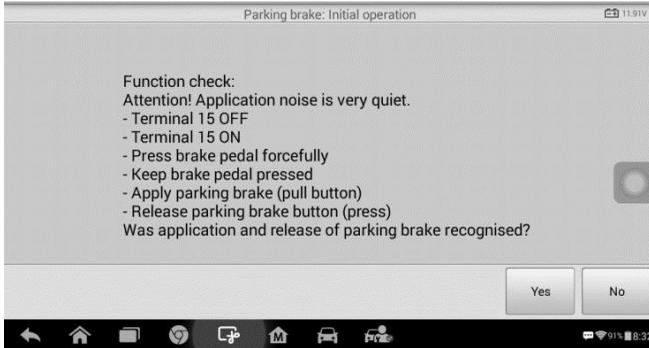
**Figure 5-7 Sample Parking brake: Initial operation Screen 1**
