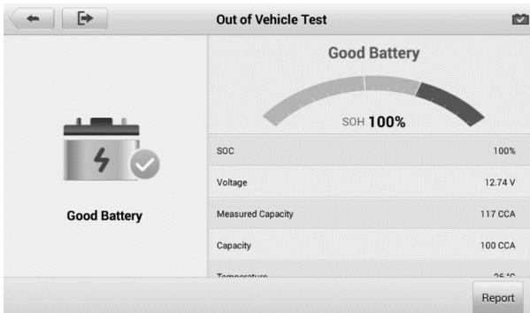
**Figure 7-12 Sample Out of Vehicle Test Results Screen**
