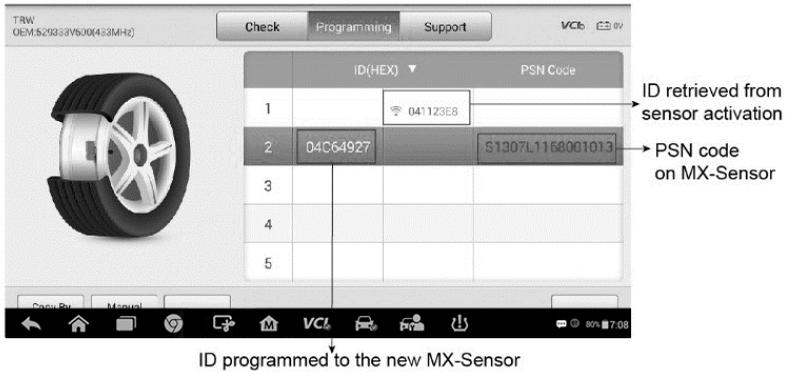
**Figure 6-34 Sample Programming Screen via OEM Part No.**
