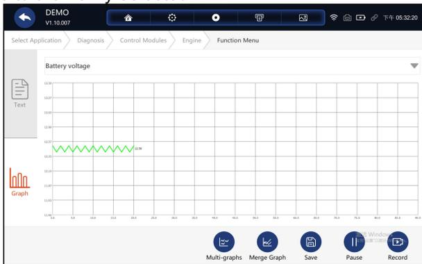
Figure 5-17 Sample PID Graph Screen
