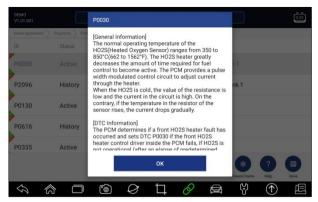
Figure 5-14 Sample DTC Help Screen
