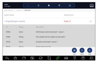
Figure 5-4 Sample Quick Scan Complete Screen
