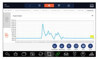
Figure 5-20 Sample PID Graph Screen
