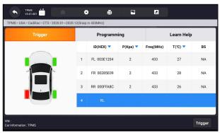
Figure 11-4 Sample Trigger TPMS Screen
