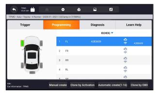
Figure 11-9 Sample Clone by Activation Function Screen
