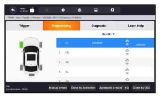
Figure 11-8 Sample Manual Create Function Screen
