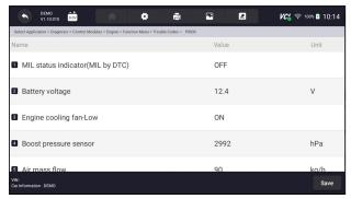
Figure 9-11 Sample Freeze Frame Screen
