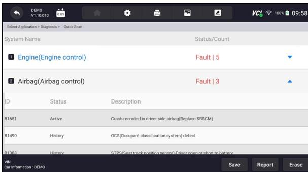
Figure 5-3 Sample Quick Scan Complete Screen
