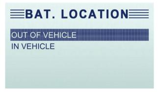
d) Scroll with the UP or DOWN button to highlight OUT OF VEHICLE or IN VEHICLE from BATTERY LOCATION menu and press ENTER to select the battery location.
