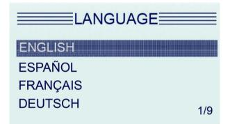
Use the UP or DOWN button to select the language you need and press the ENTER key to confirm and return. Or press ESC button to return.
