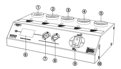
1-Standard test hole; 2-3-4-5-test hole; 6-Display screen; 7-RPM "+"; 8-RPM "-"; 9-Power switch; 10-Power port.
