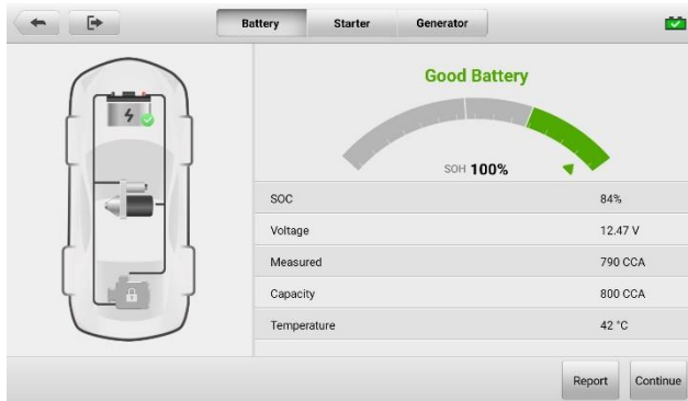
Figure 6-7 Sample Battery Test Results Screen
