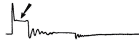
Spark plug gap is too large or mixture gas is too lean
