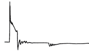
Secondary circuit resistance is too large
