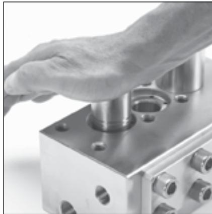
2.10 Position V/P cylinder assembly into IMDM and hand press into place.
