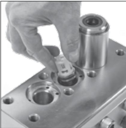
2.9 Place new assembled inlet valve assembly into each valve chamber.
