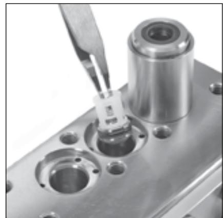
2.7 Use a reverse pliers to grasp spring retainer and pull inlet valve assembly from each valve chamber.
