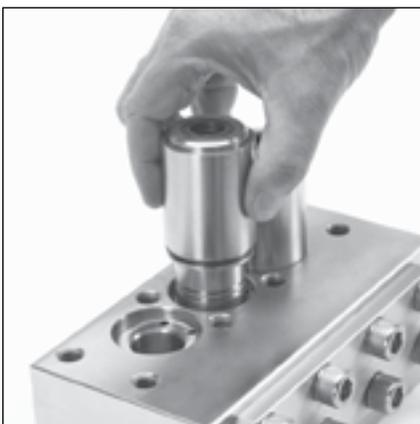
3.5 Remove outer cylinder with seal case assembly from IMDM.
