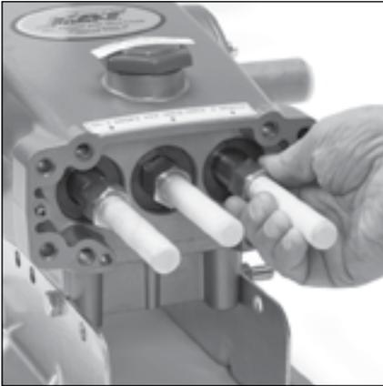
4.4 Install plunger assembly onto each plunger rod.
