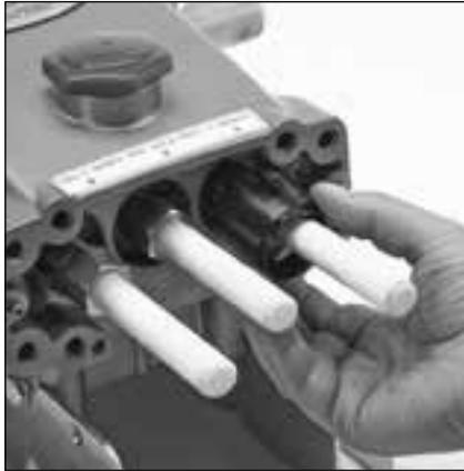
4.1 Remove seal retainers from crankcase.
