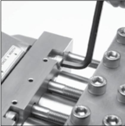
3.0 Use a M8 Allen Wrench to remove the four (4) Hex Socket Head Screws (HSH) that secure the housing block to the crankcase.
