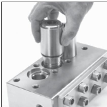
2.5 Remove outer cylinders with seal case assembly from IMDM.
