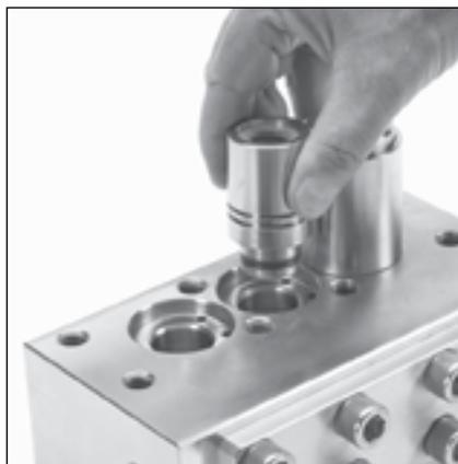
2.6 Remove V-Packing (V/P) cylinder assembly from each IMDM valve chamber.
