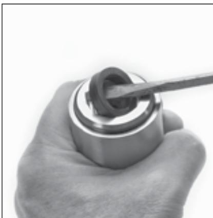
3.6 Remove low pressure seals and o-rings from each seal case.
