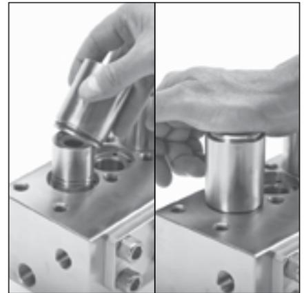
2.11 Slide outer cylinder with seal case assembly and hand press into place.
