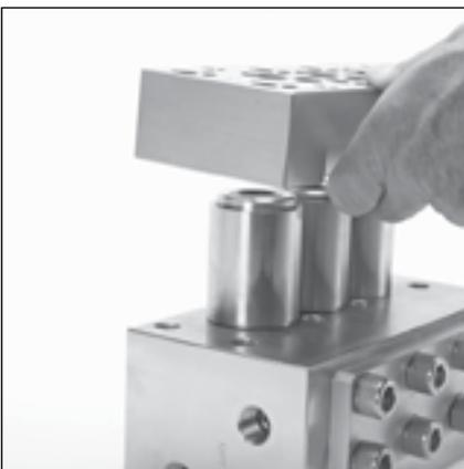
2.12 Position housing block with counter-bore surfaces facing downward over outer cylinders.
