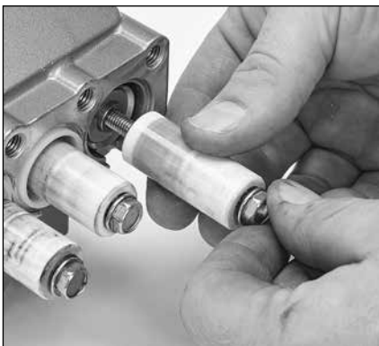
1.29 Thread plunger assembly into plunger rod by hand, and torque to 55 in-lbs, 4.6 ft-lbs or 6.2 Nm.
