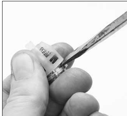
2.06 Place flat tip screwdriver in gap between valve seat and spring retainer, and twist to completely separate.
