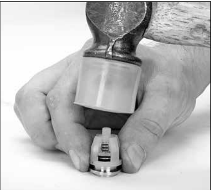
2.16 Using a rubber mallet, lightly tap spring retainer into place.
