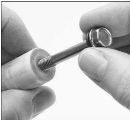
1.27 Insert plunger retainer with gasket into non-stepped side of plunger.
