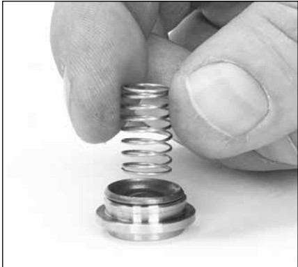
2.14 Place spring onto concave side of valve.
