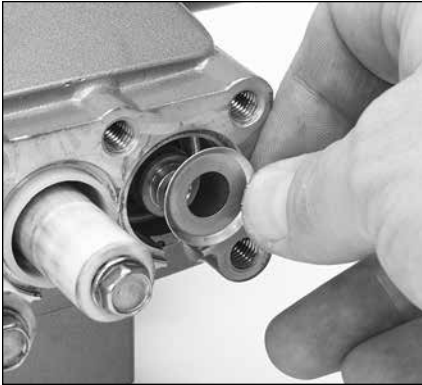
1.23 Install barrier slinger with dish side facing away from crankcase.
