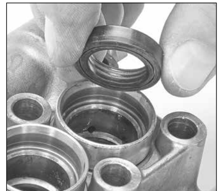
1.17 One side of the low-pressure seal has a groove and spring. Install groove side facing down and press into place.
