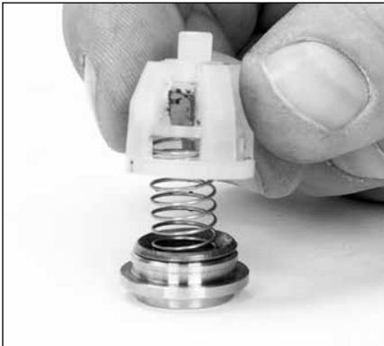
2.15 Place spring retainer onto valve seat.
