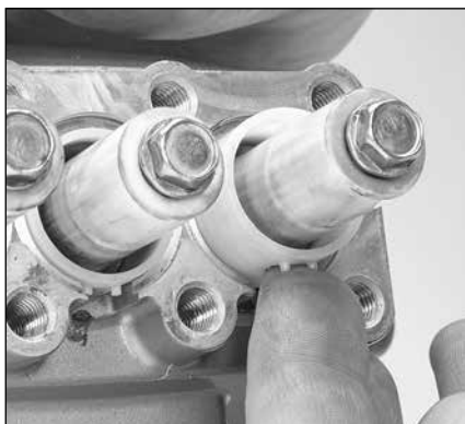
1.18 Remove seal retainers from crankcase housing.
