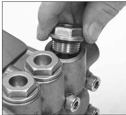
2.22 Install valve plug into manifold and thread by hand.
