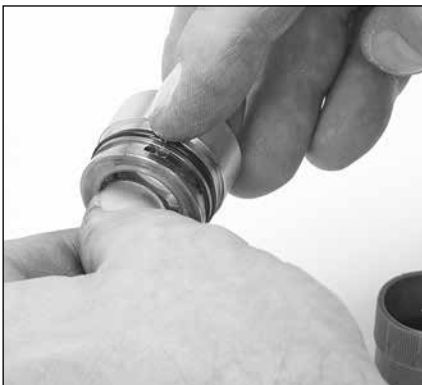
1.15 Replace seal case O-ring with new one from seal kit and apply a lubricant to outside surface.
