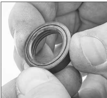
1.07 Inspect the inside diameter of the low-pressure seals for wear or damage.
