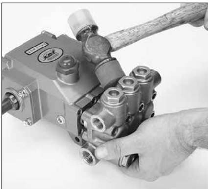
1.04 Support the manifold from underneath. Using a rubber mallet, tap the manifold to separate from the crankcase and remove completely.
