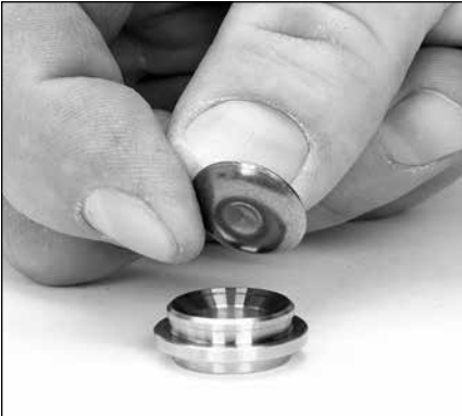
2.13 Place valve onto valve seat with tapered surface facing down.
