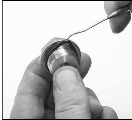
2.19 Remove old valve plug O-ring with a pick, or small flat tip screwdriver.
