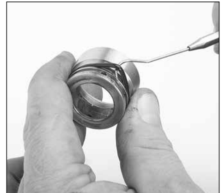
1.14 Remove seal case O-ring with a pick, or small flat tip screwdriver.
