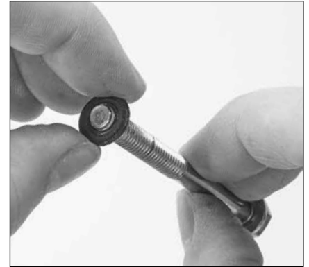
1.25 Replace plunger retainer gasket with new one from seal kit.
