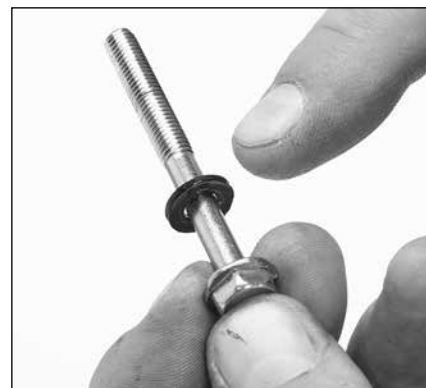
1.20 Remove and inspect plunger retainer gasket.
