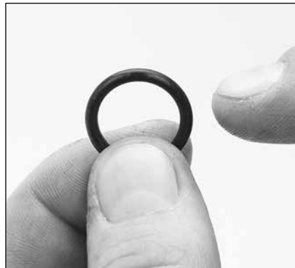
2.11 Inspect valve seat O-ring for cuts, nicks, or damage.
