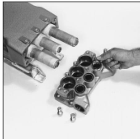
Removing the Inlet Manifold O-Ring
