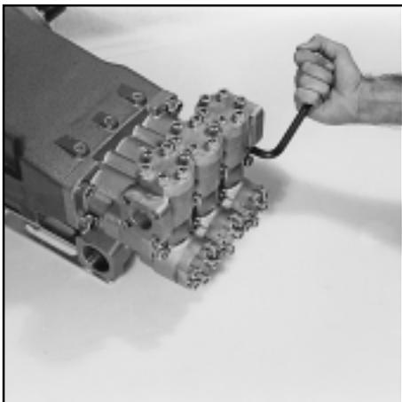
Removing Discharge Manifold screws
