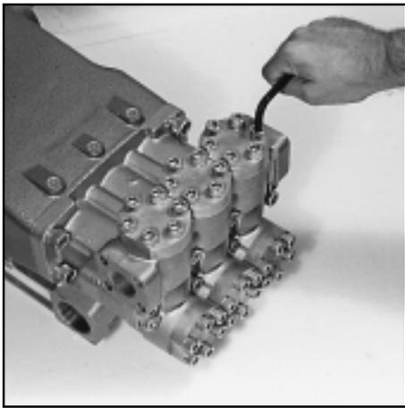
Removing Valve Plug screws
