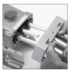
3.24 Slide complete head assembly carefully over ceramic plungers until flush against crankcase.
