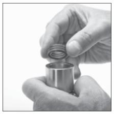
3.15 Lubricate and install v-packings with v-grooved side down into each V/P cylinder. Each cylinder requires three (3) v-packings.
