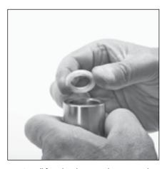
3.16 Install female adapter with v-grooved side facing down into each V/P cylinder.
