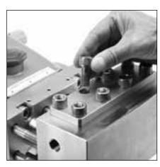
1.11 Apply anti-sieze lubricant (PN 6119) to threads of all eight (8) HSH screws and hand tighten.
