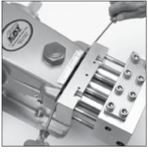
2.1 Postion two flat tip screwdrivers on either side of housing block and pry the housing block from the crankcase.
