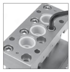
3.3 Use a M10 Allen Wrench to remove the eight (8) HSH screws that secure the housing block to the IMDM.
