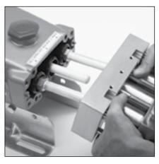
2.14 Slide complete head assembly carefully over ceramic plungers until flush against crankcase.
