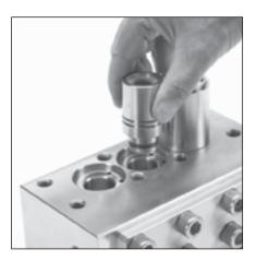
Remove V-Packing (V/P) cylinder assembly from each IMDM valve chamber.
