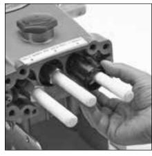
4.1 Remove seal retainers from crankcase.
