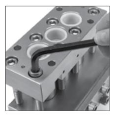
2.13 Use a M10 Allen Wrench to torque all eight (8) HSH screws to 398 in lbs, 33 ft lbs or 45 Nm in sequence show.
