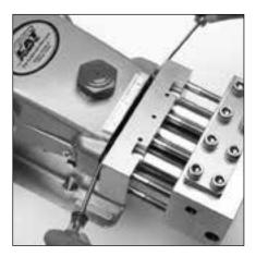
4.0 Remove IMDM and housing block as a complete assembly.
