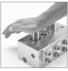
3.17 Lubricate and install backup-ring and then o-ring onto small end of each V/P cylinder. Position small end of each V/P cylinder into the IMDM and press into place.
