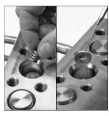
1.8 Place washer over tip of spring retainer and then coil spring.
