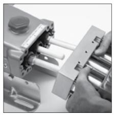
2.2 Pull complete head assembly carefully over ceramic plungers and place on a flat surface with the housing block side facing upwards.
