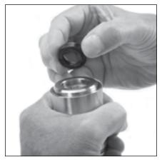
3.19 Lubricate outside diameter of each low pressure seal and inside diameter of each seal case. Install low pressue seal with spring side down into each seal case.
