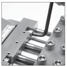
Use a M8 Allen Wrench to remove the four
