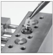
1.5 Use a needle nose pliers to grab the tip end of the spring retainer and pull valve assembly from each valve chamber.
