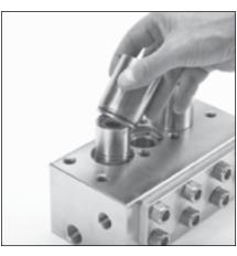
3.18 Lubricate and install o-ring into groove of each outer cylinder. Slide outer cylinder over each V/P cylinder and hand press into IMDM.
