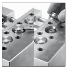
1.2 Use a flat tip screwdriver to remove valve plugs from each valve chamber.
