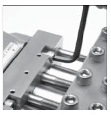
4.8 Use a M8 Allen Wrench to torque all four(4) HSH screws to 531 in lbs, 44 ft lbs or 60Nm in sequence show.
