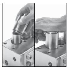
2.11 Slide outer cylinder with seal case assembly and hand press into place.
