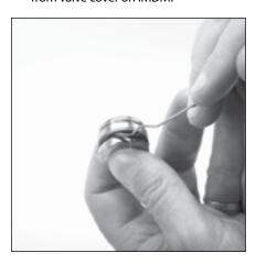
1.3 Use a pick tool to remove backup-ring and o-ring from each valve plug.
