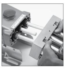
4.7 Slide complete head assembly carefully over ceramic plungers until flush against crankcase.
