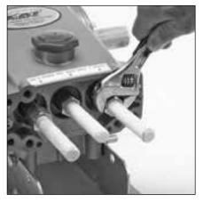
4.2 Use a 7/8" wrench to remove plunger assembly from each plunger rod.
