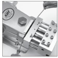
3.1 Postion two flat tip screwdrivers on either side of housing block and pry the housing block from the crankcase.
