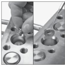
1.4 Remove coil spring and then washer from each valve chamber.
