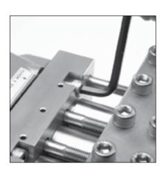
2.15 Use a M8 Allen Wrench to torque all four (4) HSH screws to 531 in lbs, 44 ft lbs or 60 Nm in sequence show.
