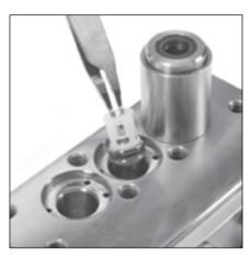
2.7 Use a reverse pliers to grasp spring retainer and pull inlet valve assembly from each valve chamber.
