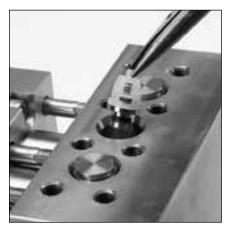
1.7 Place new assemblied discharge valve assembly into each valve chamber.
