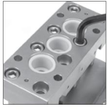
2.3 Use a M10 Allen Wrench to remove the eight (8) HSH screws that secure the housing block to the IMDM.
