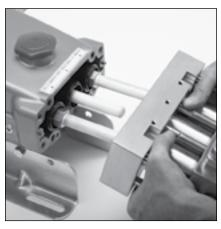
3.2 Pull complete head assembly carefully over ceramic plungers and place on a flat surface with the housing block side facing upwards.
