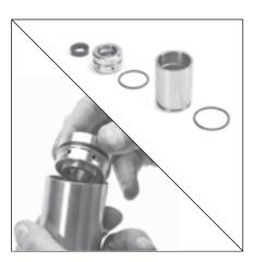
3.7 Remove seal case assembly from each outer cylinder.
