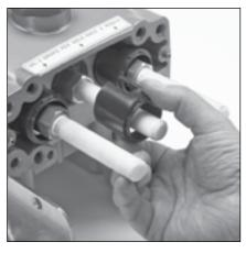
4.6 Install seal retainers with slot opening facing upwards and the small stepped diameter facing the manifold.
