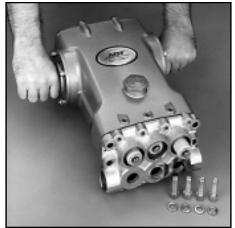
Rotate Crankshaft to position plungers
