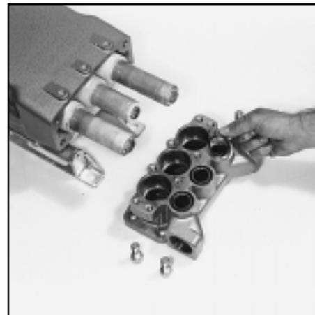
Removing the Inlet Manifold O-Ring
