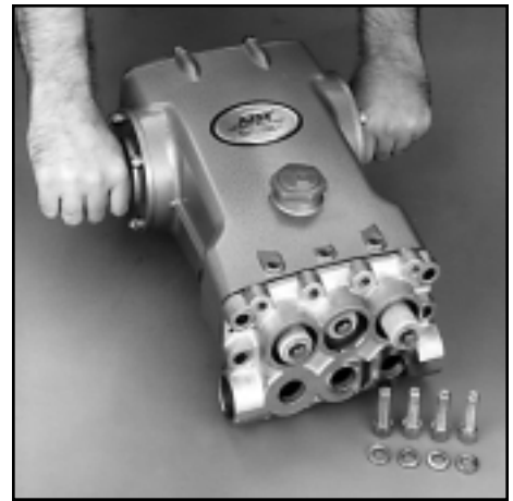
Rotate Crankshaft to position plungers
