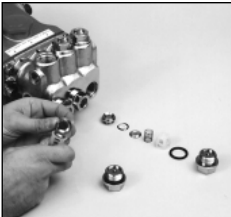
Order of parts in Valve Assembly
