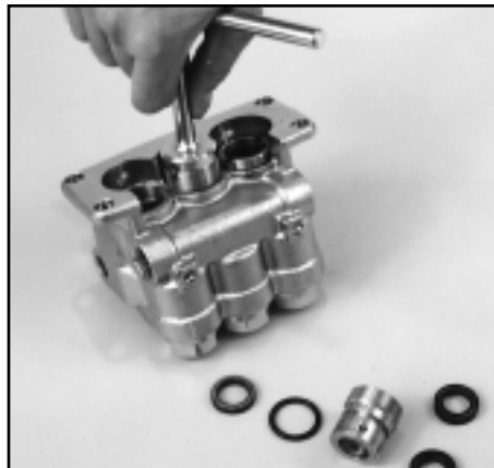
Removal of Seal Cases from Manifold Head
