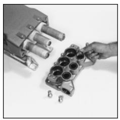
Removing the Inlet Manifold O-Ring
