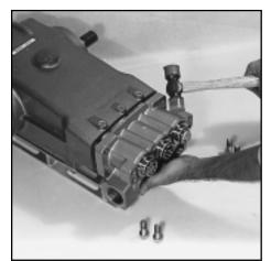
Removing the Discharge Manifold
