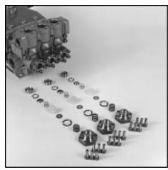
**Removing Valve Plug screws**
