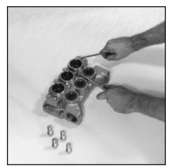
Removing the V-Packing Cylinder
