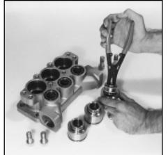
Removing the V-Packing Spacer from the Cylinder
