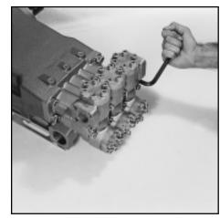
**Removing Discharge Manifold screws**
