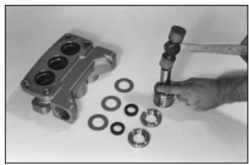
Removing the Inlet Adapter from the Inlet Manifold
