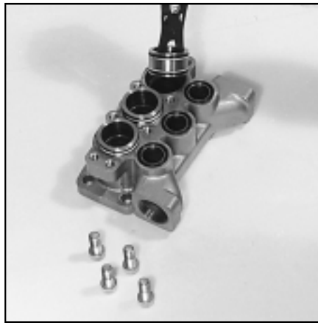
3531, 3535, 3537, 3541, 3545, 3650 Removal of V-Packing Spacer from Inlet Manifold
