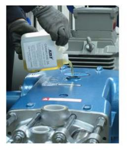
Good lubrication is the simplest, most efficient and least expensive preventative maintenance for your pump. Use only genuine/approved Cat Pumps crankcase oil to extend the life of your high pressure reciprocating pump.
