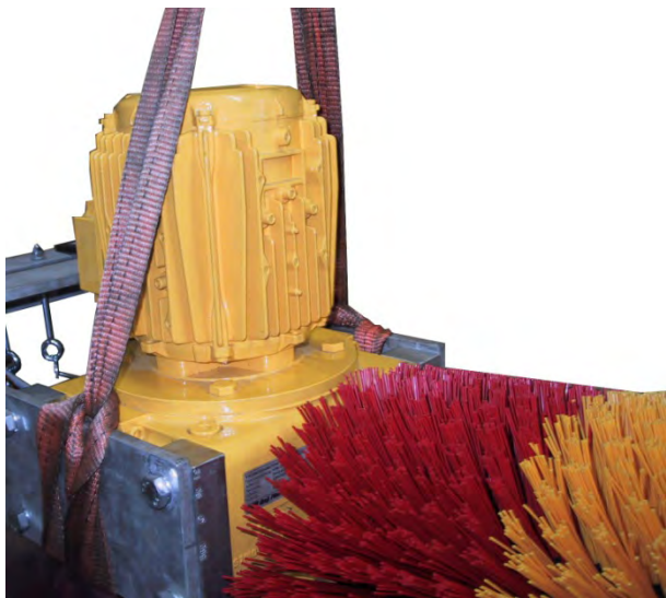
Figure 3: Affixing the lifting harness
