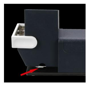
The Signoscope is adjusted from the factory for normal stamp thickness. In exceptional cases, the position lever must be readjusted for extremely thin or extremely thick stamps.
