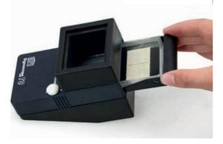
Lift the projection glass and place the stamp between the plexiglass and the metal plate. When examining watermarks, place the stamp face down in the center of the slide.
