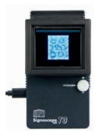
The intensity of the light source is adjusted by moving the control knob up (brighter) or down (darker).
