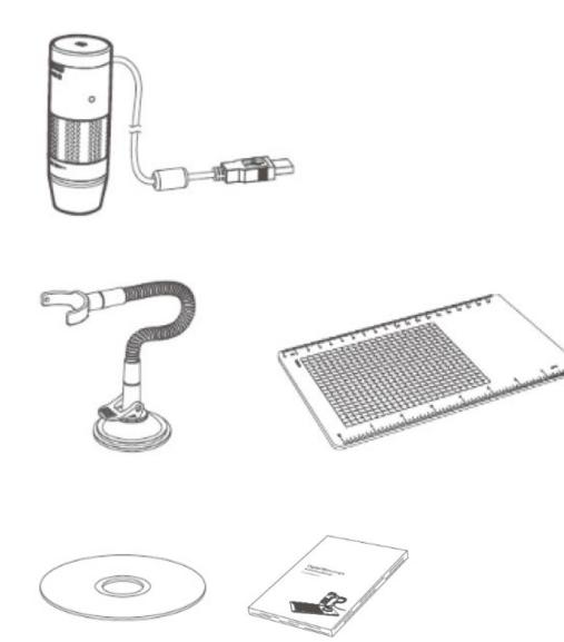
USB Microscope Holder with suction cup Gridded footplate Installation CD Directions for use
