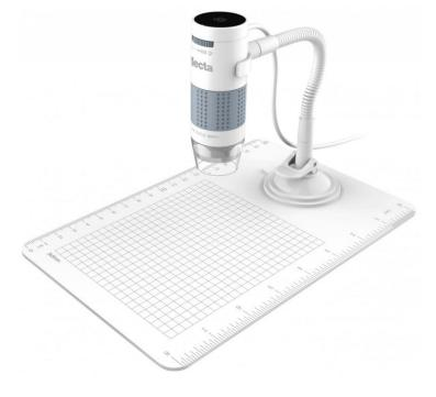
Specification Connection type USB 2.0 Effective magnifications (on a 17" screen) 60x, 250x Effective display area 5.6 x 4.2 mm (60x), 1.4 x 1.1 mm (250x), Lighting Four LED lights Power supply 5V 250mA (via USB) CMOS sensor Maximum resolution snapshot 1600 x 1200 pixels (UXGA) Maximum video recording resolution 640 x 480 pixels (VGA) Dimensions  $\Phi$  30 x 86 mm Weight 207 grams Net weight of product: 250 g
