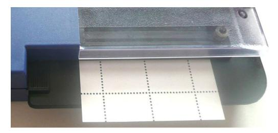
Place the back of the stamp facing up, because the optical reader has the most ideal reading ability between the back of the stamp usually white/yellow and the perforation hole which is considered black. If the stamp is face up, this could affect the quality of reading. Examination of larger stamps and roll stamps is also possible, provided they come correctly against the stop. The stop is open on the right side.
