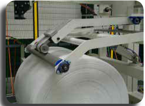
Nip roller: Low resistance torque to avoid any problem when winding sensitive products
