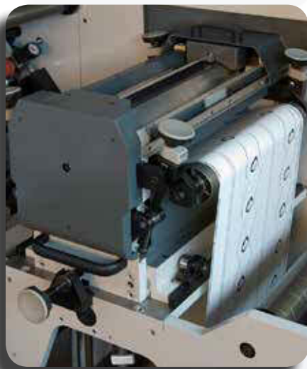
ALVEOTUBE® with helically grooves and hard anodised, used on a printing machine
