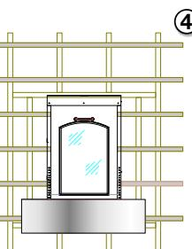
Now install the casement stay (included separately in the package). Slide the casement stay straight into the opening of the eye without twisting.
