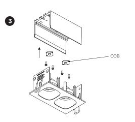
DISMOUNTING INSTRUCTION Light Source Take the luminaire out of the ceiling hole and disconnect the wires. Remove the side screws. Take everything apart to remove the COB Module. To replace the light source please contact your Wever & Ducré customer service contact point.
