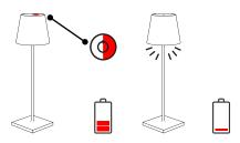
FLASHING RED LED the battery charge is lower than 20%, charging is recommended. When the charge is depleted (1%), the lamp does not switch on but emits three white flashes as an alert to charge
