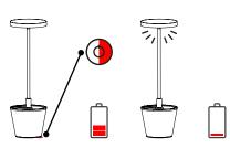
FLASHING RED LED the battery charge is lower than 20%, charging is recommended. When the charge is depleted (1%), the lamp does not switch on but emits three white flashes as an alert to charge
