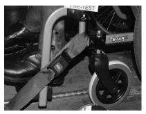
Fitting the front restraint
