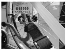
Fitting the rear restraint
