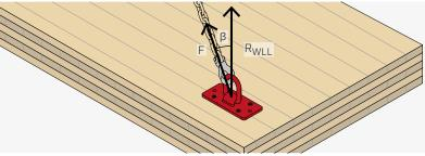
NOTE:  $\beta$  = lifting angle (angle between vertical axis and chain).
