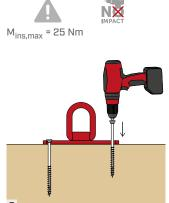
Length and quantity of screws depend on the type of application. Drive the screws in the holes provided, being careful not to overtighten them.
