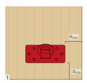
Read the instructions for use carefully and follow the directions. The positioning of the plate on the timber element must comply with the minimum distances.
