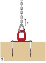
Connect the crane hook and carefully lift the timber element. Be careful about the allowed lifting directions and corresponding maximum lifting capacities.
