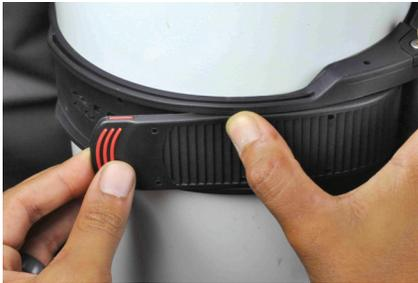
Tuck excess tank band into recess channel
