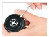
Use a small screwdriver to carefully remove the Locking Ring. Press towards the center of the lid to release it from the groove, then slightly press upwards.
